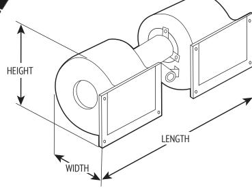
Use the diagram above as a reference to measure the dimensions of your blower. This will help you determine which is suitable for your vehicle.
