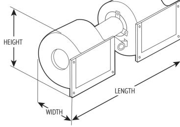
Use the diagram above as a reference to measure the dimensions of your blower. This will help you determine which is suitable for your vehicle.
